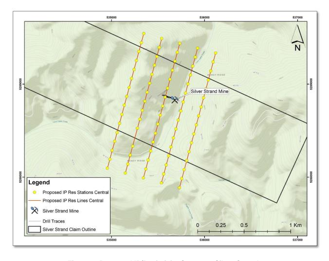
Figure 1. Proposed IP/Resistivity Survey at Silver Strand
