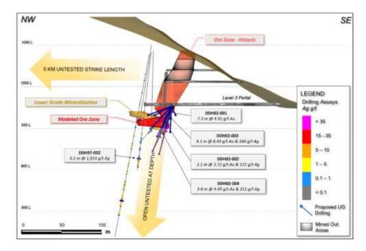
Figure 1. Non-NI 43-101 Compliant model showing proposed Phase I underground drilling.<sup>1</sup>
